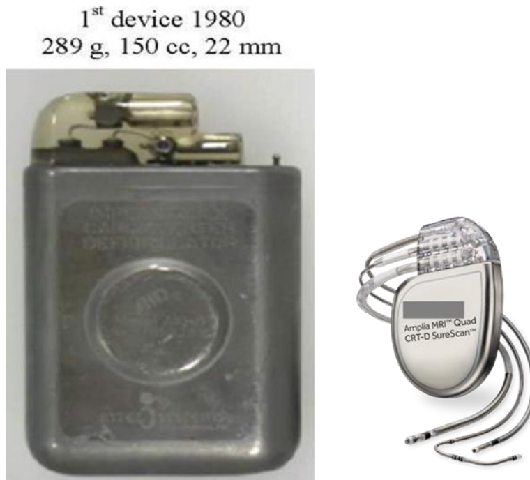
Fig. 1. Original implantable cardioverter defibrillator pulse generator, on the left, and a modern device on the right, CRT-D]
